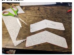
Step 5: Line up the paper template with the foam wing using the trailing edge as a reference.
