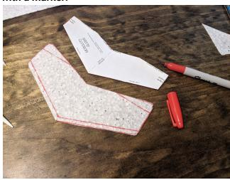
Step 7: Using the edge of a credit card, make an indentation in the foam along the folded dotted lines of the template.
