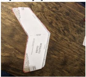
Step 2: Trace the wing shape onto a piece of foam with a marker. If you're careful, each sheet of foam can make two gliders
