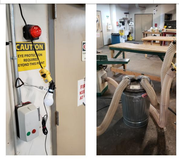
Under normal circumstances it just works. Power on a machine that has an IVAC sensor attached to its power cord, its gate will open and the vacuum gets powered. Turn off the tool, the system will run for 1 minute longer allowing for the lines to clear, but also to prevent too frequent starts and stops. If you use a remote to start the collector, that same remote must be used to turn it off. What can go wrong?
