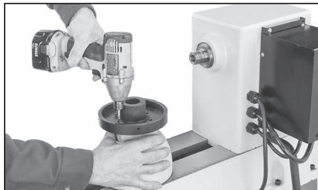
Figure 43. Typical attachment of faceplate to workpiece.
