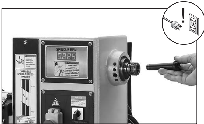
Figure 25. Installing center into the headstock spindle.
