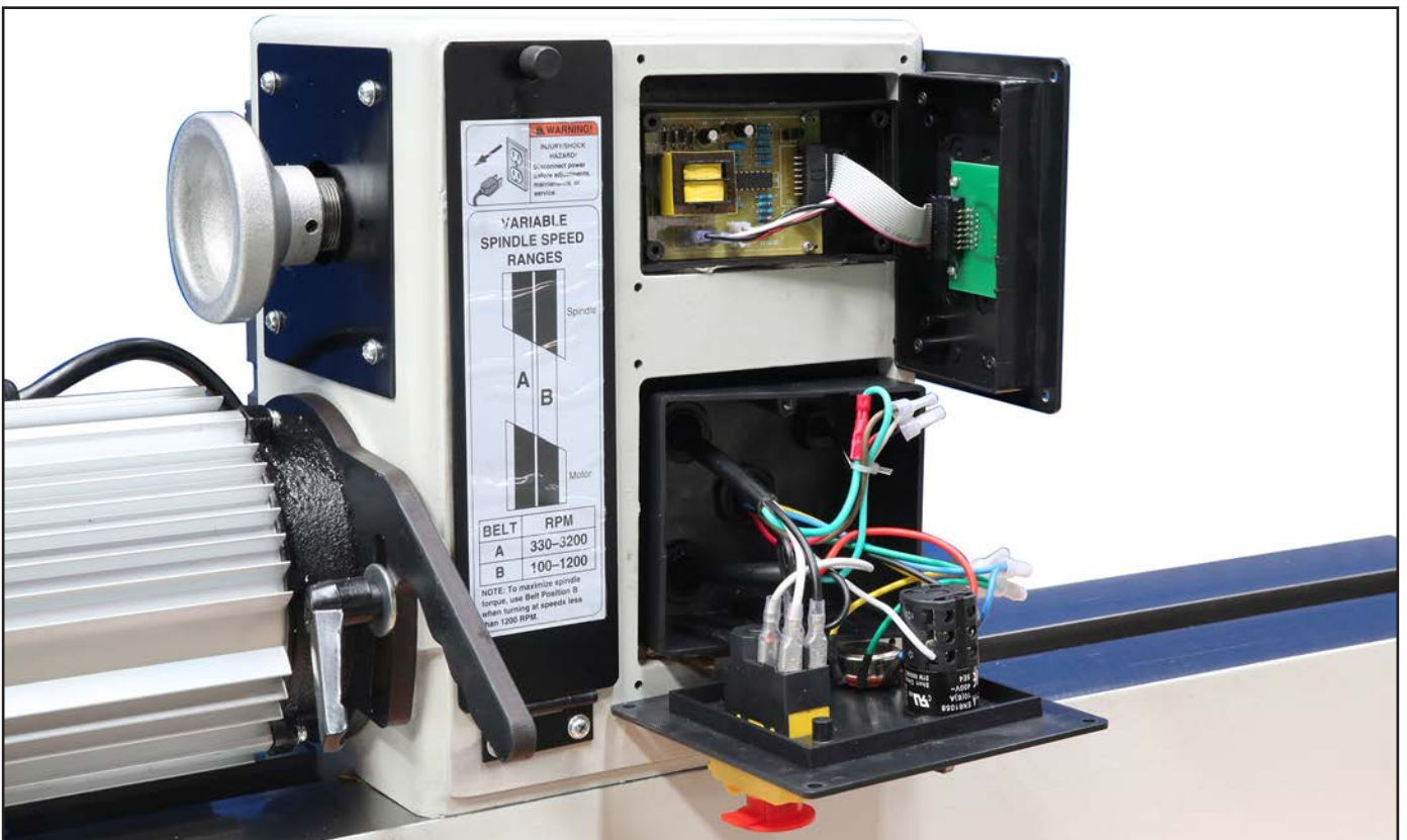
Figure 66. RPM readout display board and control panel wiring.
