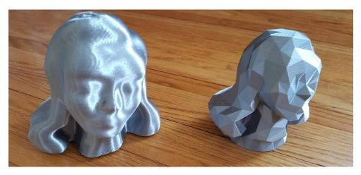
D. I believe the smaller diameter filament used increased the reflectivity and also enhanced the Moiré pattern evident on the smooth print.
