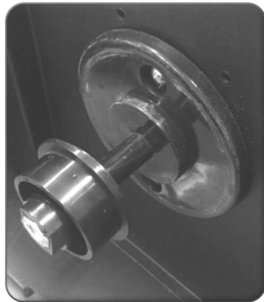
Above Image: Correct assembly of wire carrier for use with 4" spools.
