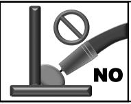
**Characteristics:** Large convex weld with bulging at toes, weld legs exceed thickness of the metal being welded.
