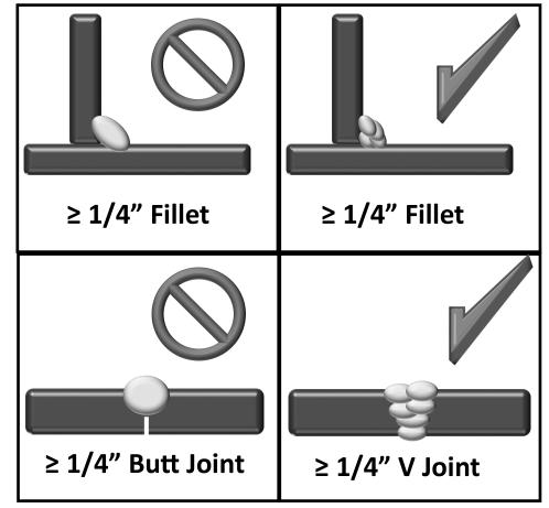
When welding material 1/4" and over be careful about trying to put too much metal down in a single pass. Use multiple passes to complete the weld along with any necessary joint preparation. As metal thickness goes up so does the number of required passes. Depending upon the wire diameter and power settings used, a 1/4" joint may only require 1 or 2 passes, but a 3/8" joint in plate metal or pipe will require not only beveling but 4 to 6 overlapping weld passes including a cap and root pass.
