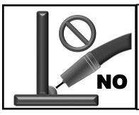
Characteristics: Small Convex weld possibly with bulging sides/cold lap and/or an inconsistent arc. Possible Causes: Not enough Voltage or Amperage. If weld is ropy and thin without bulging at the toes, travel speed is too fast or using a pull technique.
